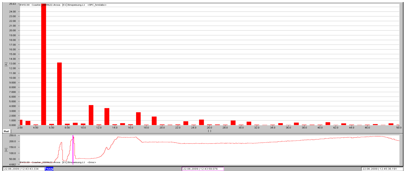
Spectrum of the harmonic currents with ECOsine™ Active (5. = 26A, 7. = 13A, 11. = 4A, 13. = 3.5A)
